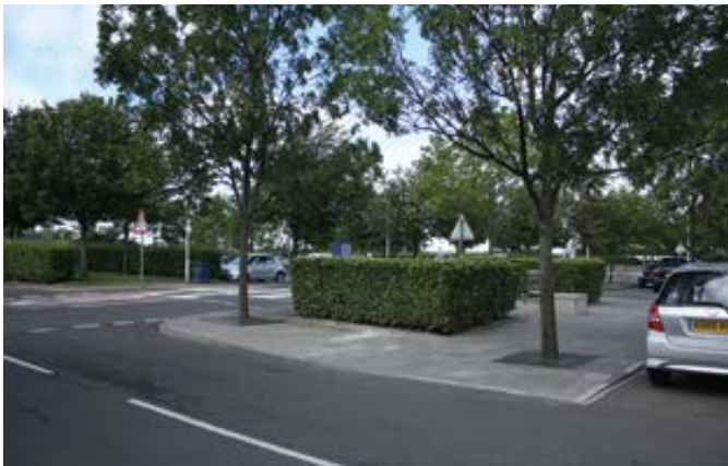
Inclusion of robust landscape with trees and hedges helps to reduce the potentially negative visual impact of the car parking area
